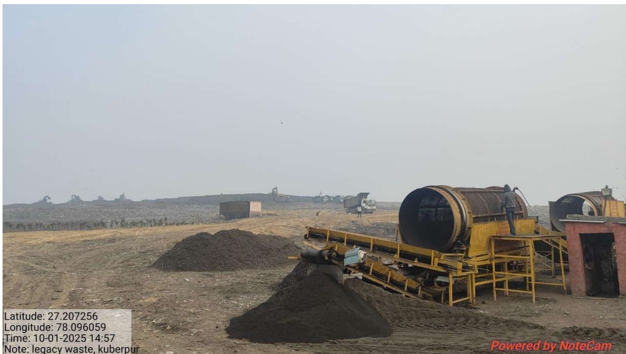
Pic.-3- Bio-mining work is in progress at Kuberpur MSW site, Agra
